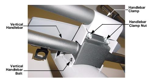
2. While supporting the vertical handlebar, remove both handlebar clamp nuts. Carefully, lower the vertical handlebar and then rotate it and set it on the left and right handlebars as shown in Diagram 10.11.2.
