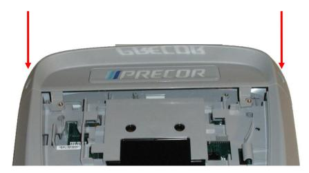
11. Remove the 6 screws that fasten the rear cover from the console and remove. **See Diagram 5.6.7.**
