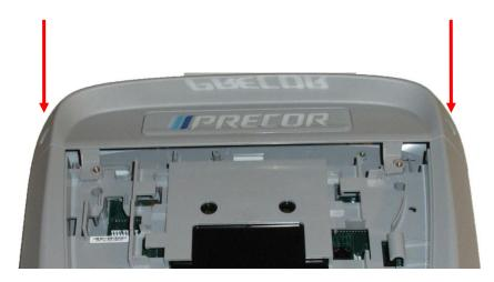
12. Remove the 6 screws that fasten the rear cover from the console and remove. **See Diagram 5.5.7.**
